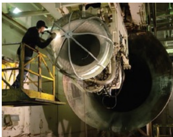
Brian McDaniel, a jet engine inspector, checks for leaks in an F118-100 engine for a B-2 Stealth Bomber in the Engine Test Cell with the 547th Propulsion Maintenance Squadron (Air Force photo by Kelly White)
