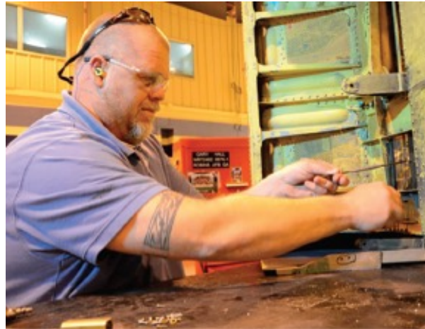
Gary Hall, 572nd Commodities Maintenance Squadron sheet metal mechanic, reinstalls an interior screen after removing foreign objects from inside an F-15 intake ramp (Air Force photo by Ed Aspera)
