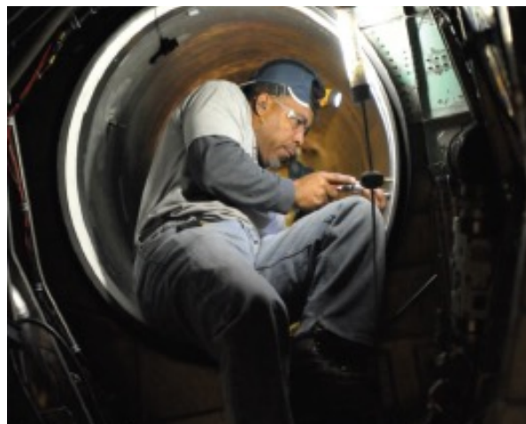
Anthony Farrow, 561st Aircraft Maintenance Squadron Production Support, changes intake fasteners on an F-15. (Air Force photo by Ray Crayton)
