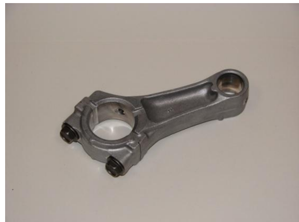
Connecting Rod: a rod that connects the piston to the crankshaft.
