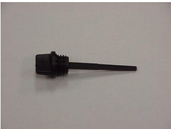
Oil Filler Plug: the device that closes the opening where the crankcase is filled with oil.
