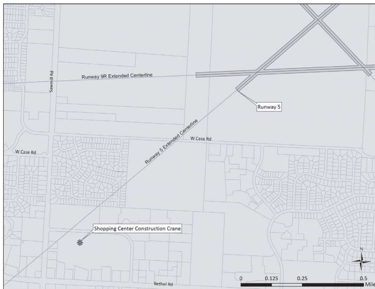
Figure D.19. A construction crane appeared one mile from the end of Runway 5. No 7460-1 Form was filed with the FAA.
