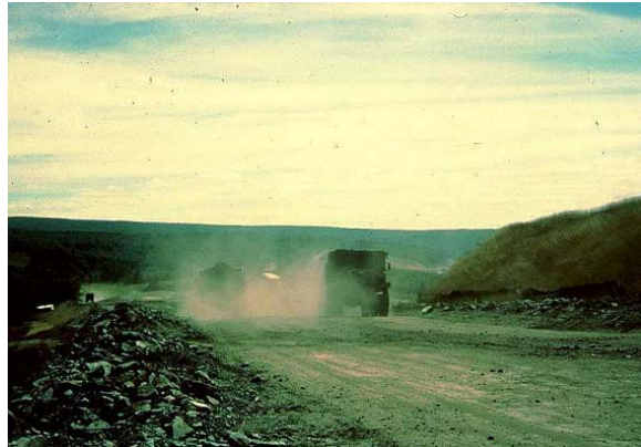
7-05 Traffic weight and speed increase dust.
