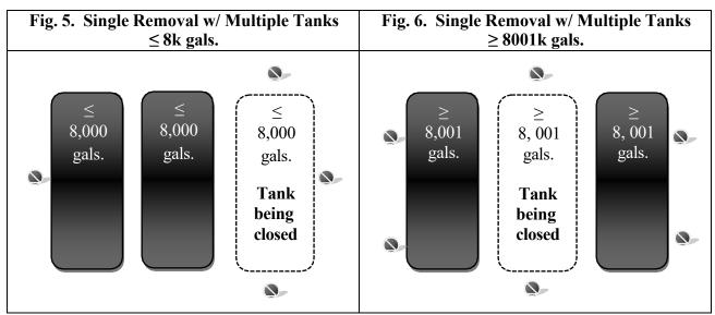
\*\* If only one (1) tank within a multi-tank pit is to be closed in-place, the sampling protocol illustrated in Figs. 5 and 6 (depending on the size of the tank) should be used to cover all four (4) sides of the tank pit. Sampling at the ends of the tank will only be required of the tank is being closed in-place.
