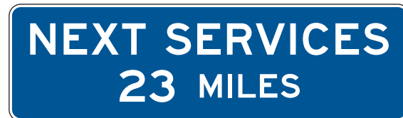
Figure 2I-2. Example of Next Services Plaque
