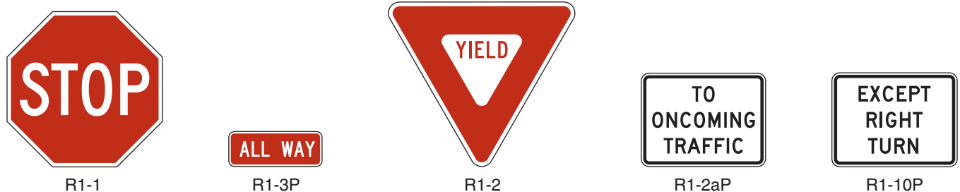
Figure 2B-1. STOP and YIELD Signs and Plaques
