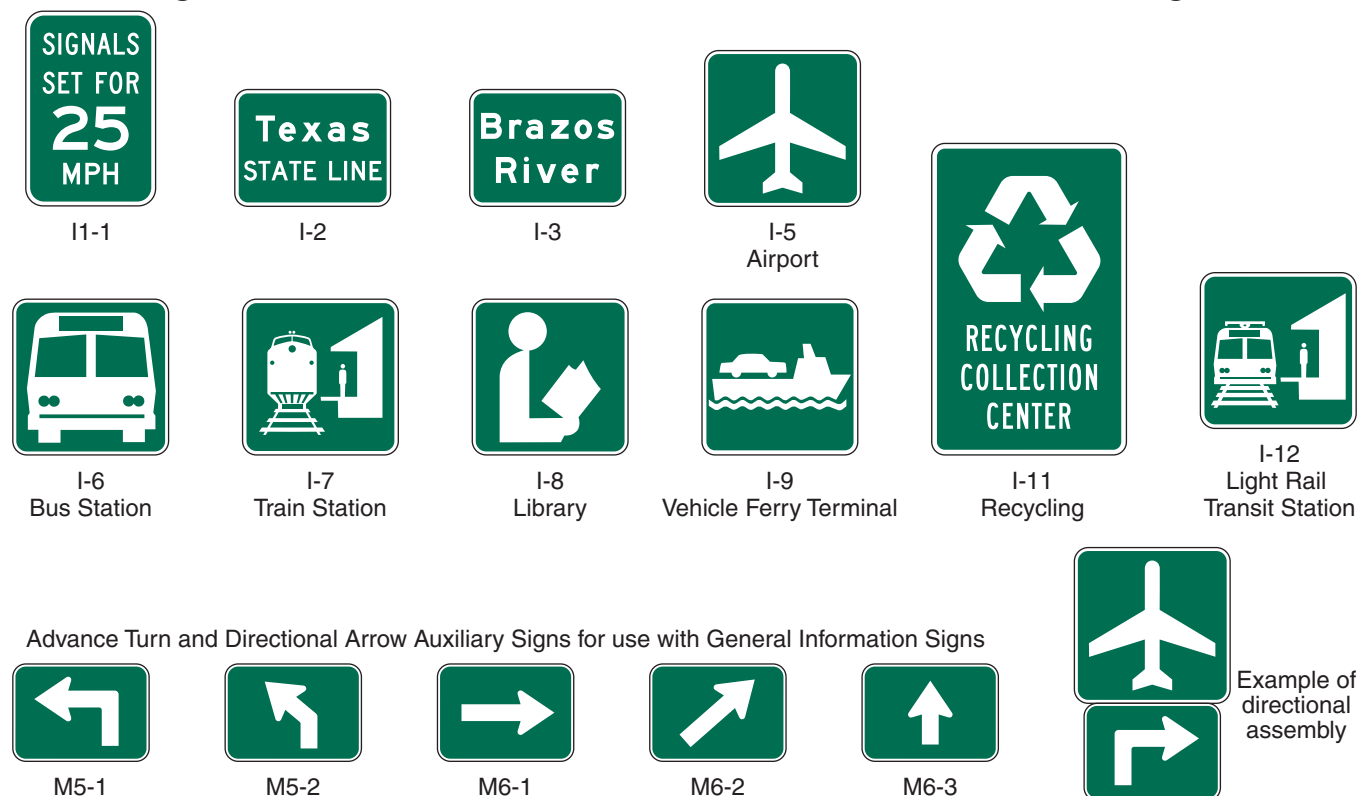
Figure 2H-1. General Information and Miscellaneous Information Signs
