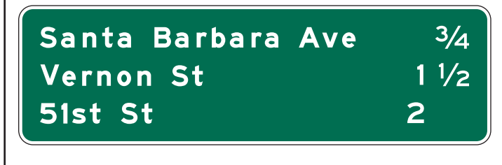
Figure 2E-31. Interchange Sequence Sign
