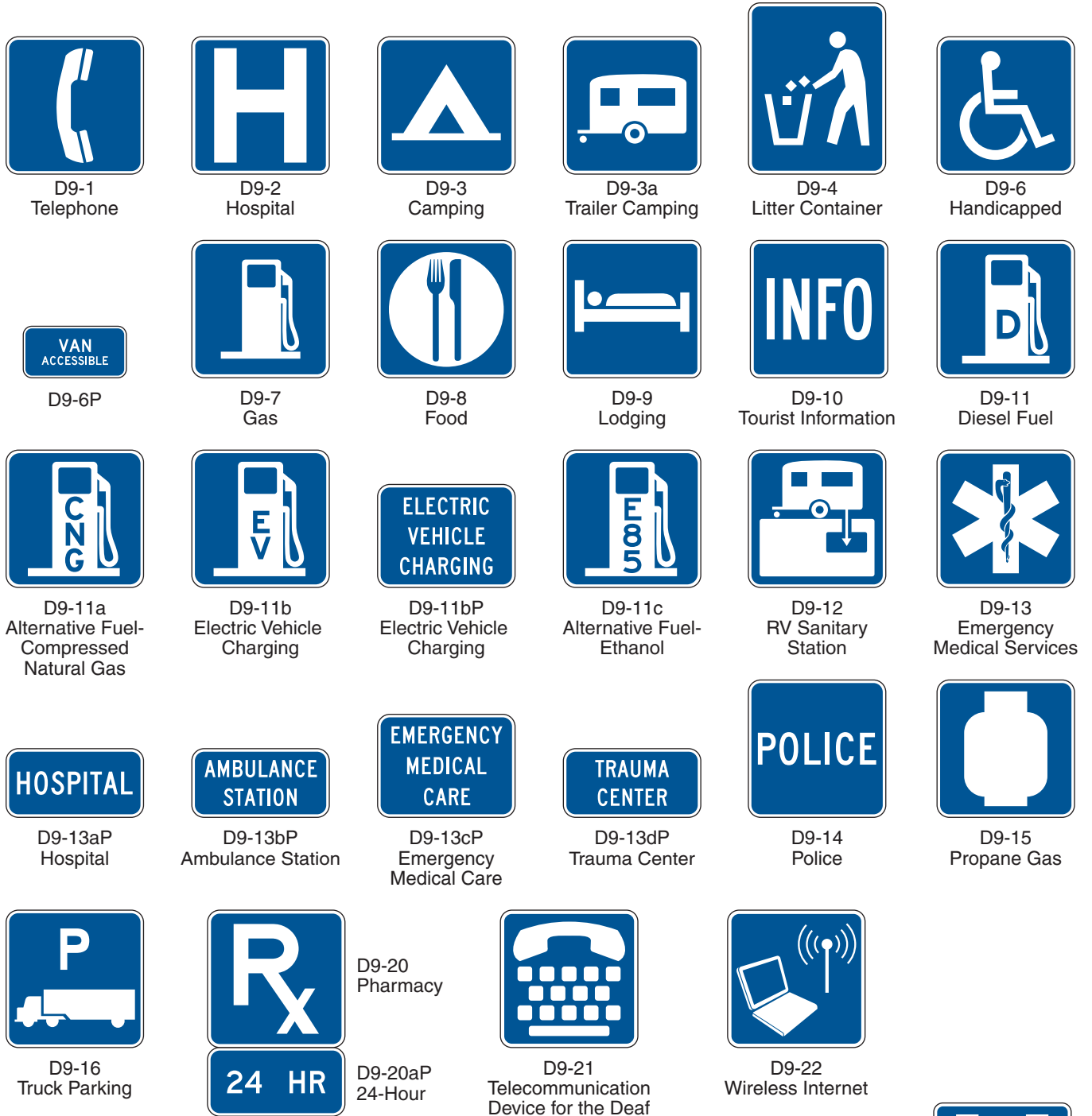
Figure 2I-1. General Service Signs and Plaques
