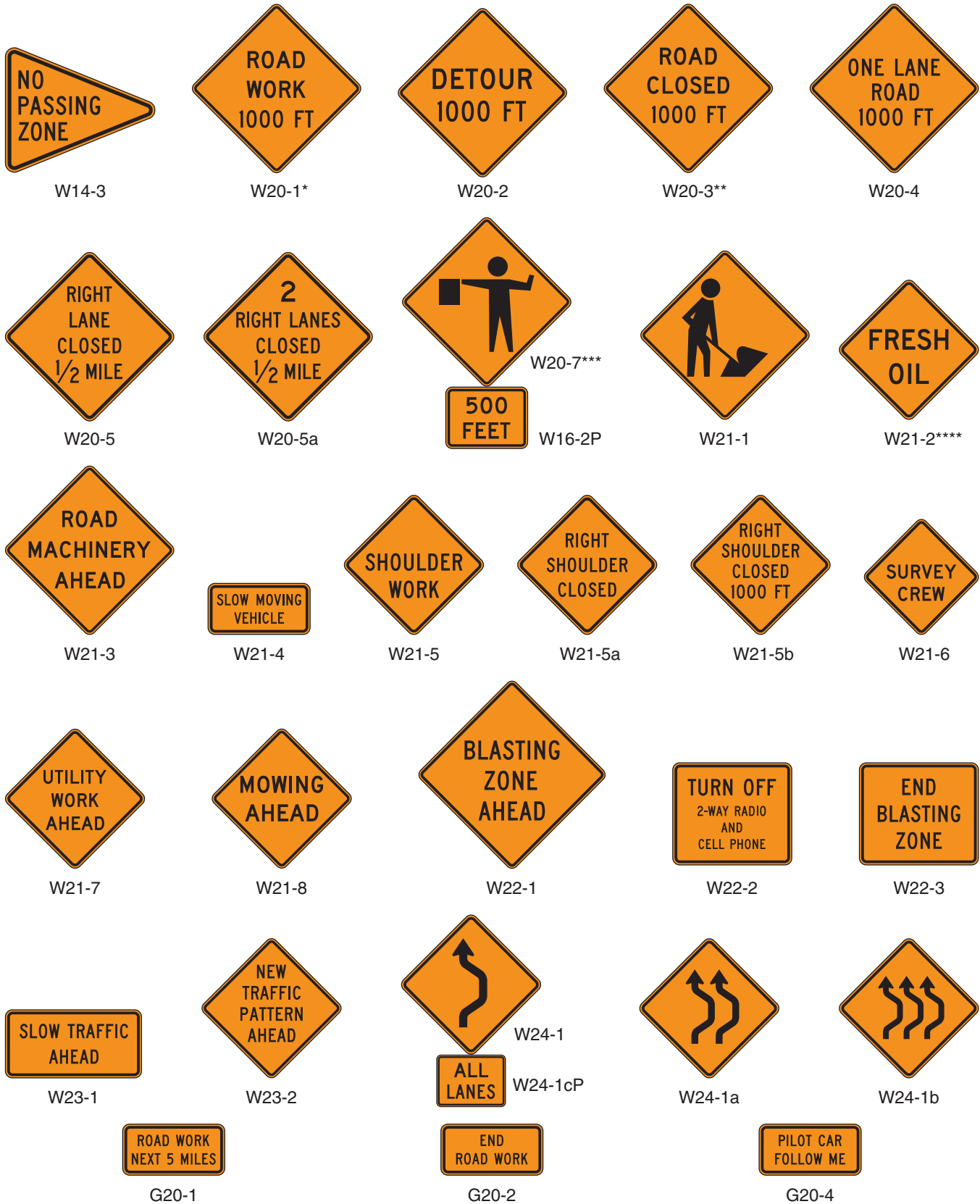
Figure 6F-4. Warning Signs and Plaques in Temporary Traffic Control Zones (Sheet 3 of 3)
