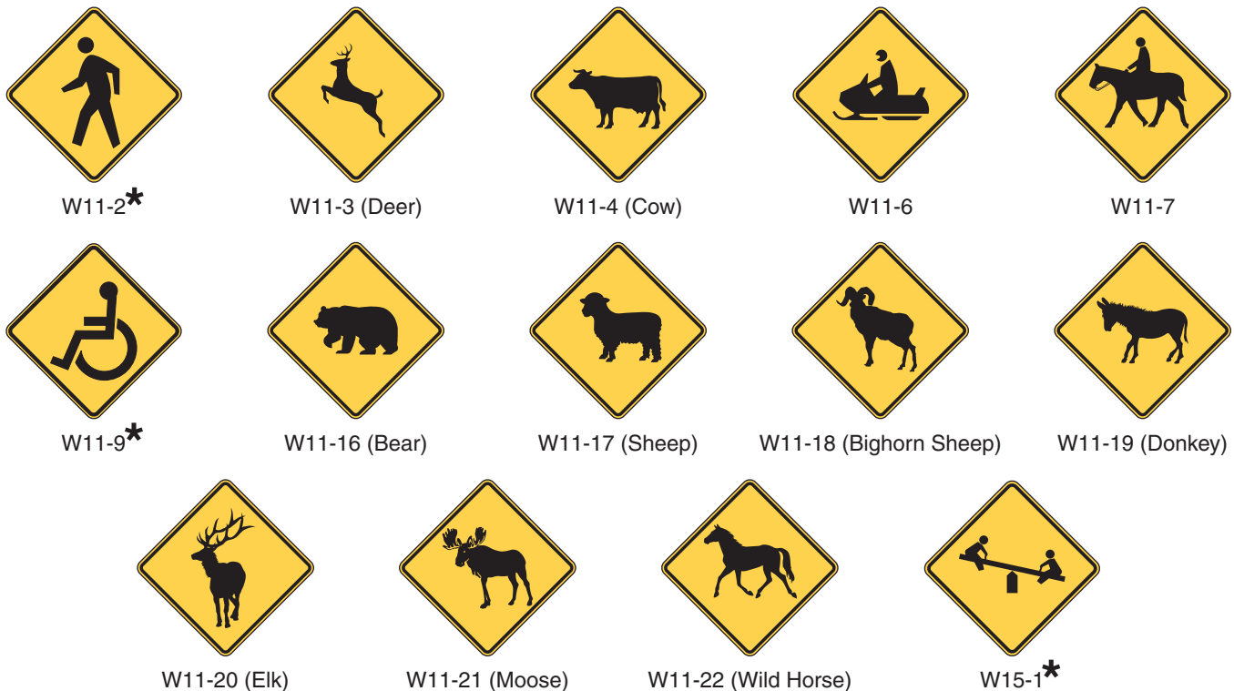
Figure 2C-11. Non-Vehicular Warning Signs
