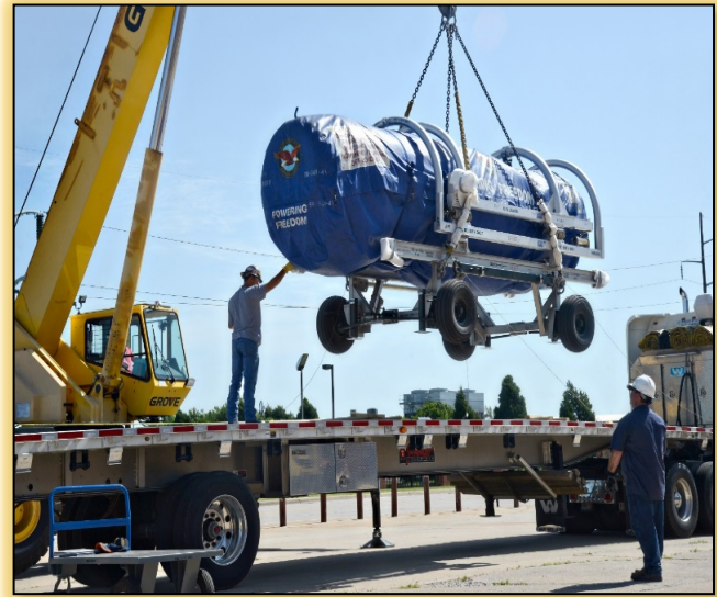
Figure 7: Shipping US Marine Corps F153 engines by truck from Tinker AFB after retrofit
