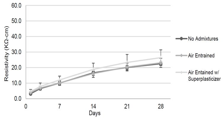
Comparison of addition of admixtures for mixtures prepared with Type I cement, 40% slag cement and 0.40 w/cm
