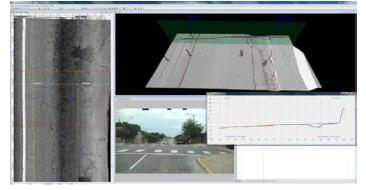
used, including the OSU 3D laser imaging technology (named as PaveVision3D Ultra, example output shown left) for 1mm 3D runway surface data, Grip Tester for continuous surface friction, dynamic friction tester (DFT) for dynamic friction coefficients, AMES high speed profiler for
