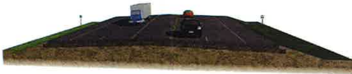
5-Lane Open Typical Section
