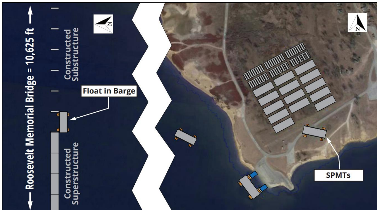
Figure 16: Example of a Float-in Modular Span Technique
