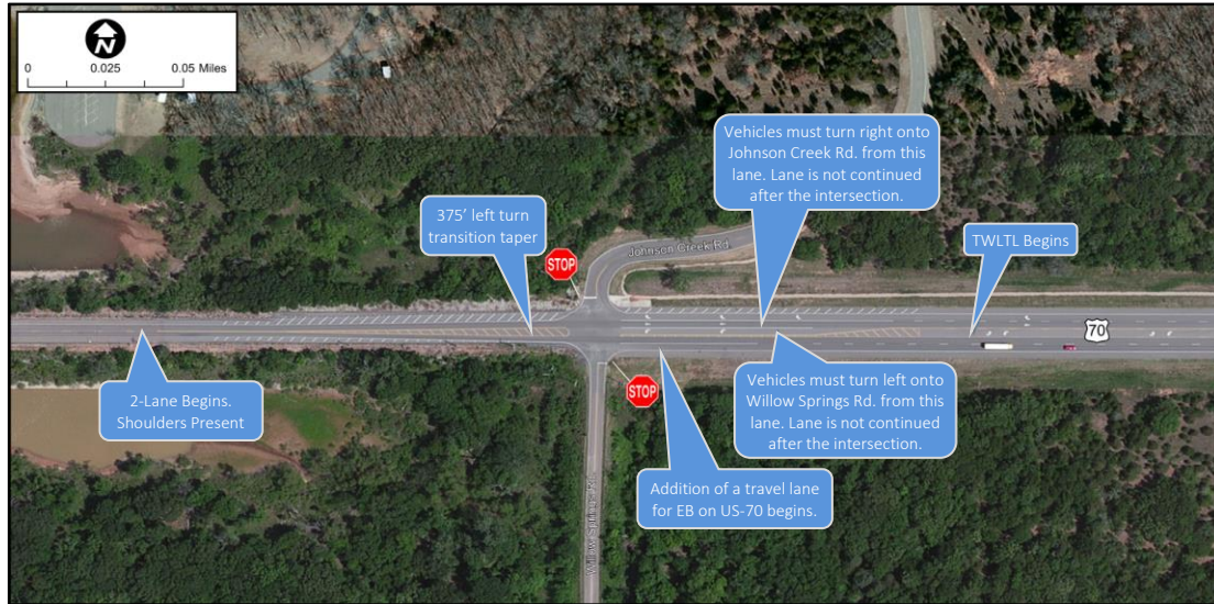
Figure 11: Segment 3 – Eastern Approach to the Bridge at Johnson Creek Road Lane Transitions
