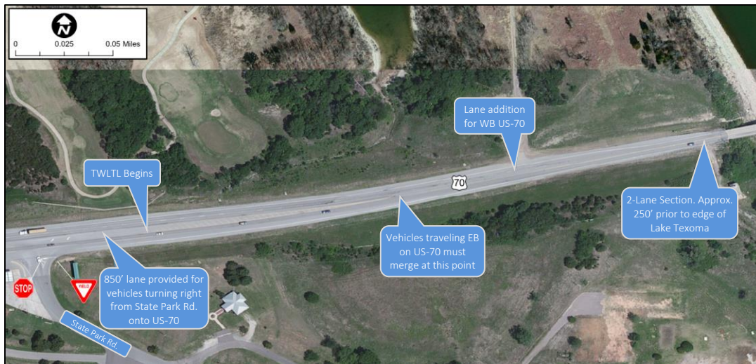
Figure 5: Segment 1 - Western Approach to Roosevelt Bridge Lane Transitions
