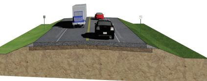
2-Lane Typical Roadway Section Typical includes: two 12-foot wide driving lanes; 8-foot wide shoulders
