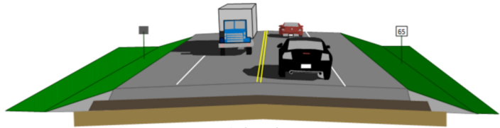
2-Lane Typical Roadway Section Typical includes: two 11-foot-wide driving lanes; 6-foot-wide shoulders
