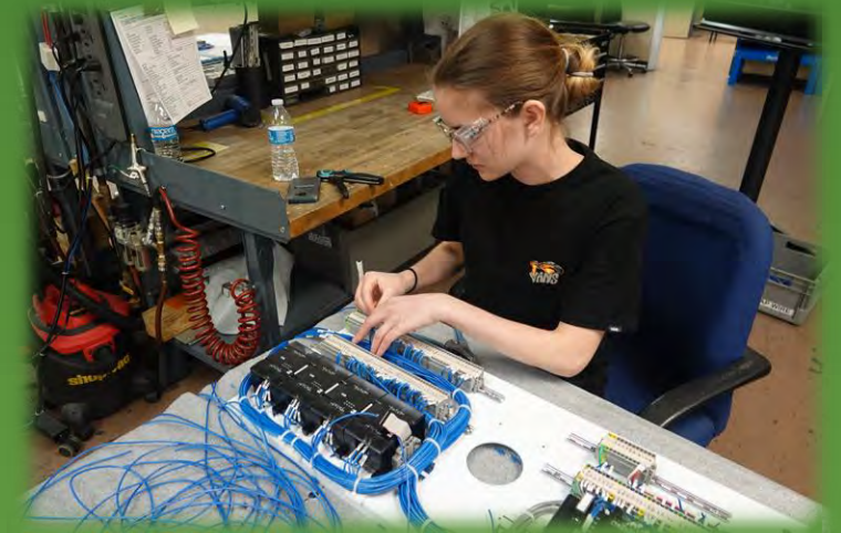
Talia wires a control panel that she helped design at HE&M Saw for a new automated carbide manufacturing center.
